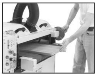
Figure 4. ALWAYS keep yourself and bystanders away from the path of potential workpiece kickback.
